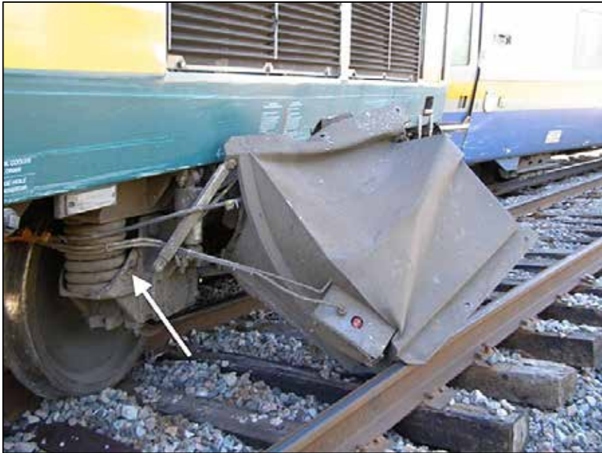
Photo 6. Impact mark on locomotive VIA 915's rear truck side frame (arrow) and separated battery box
