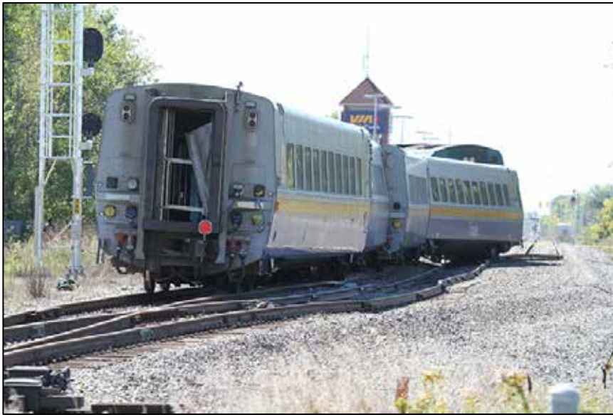
Photo 8. Westward view of derailed cars and displaced track
