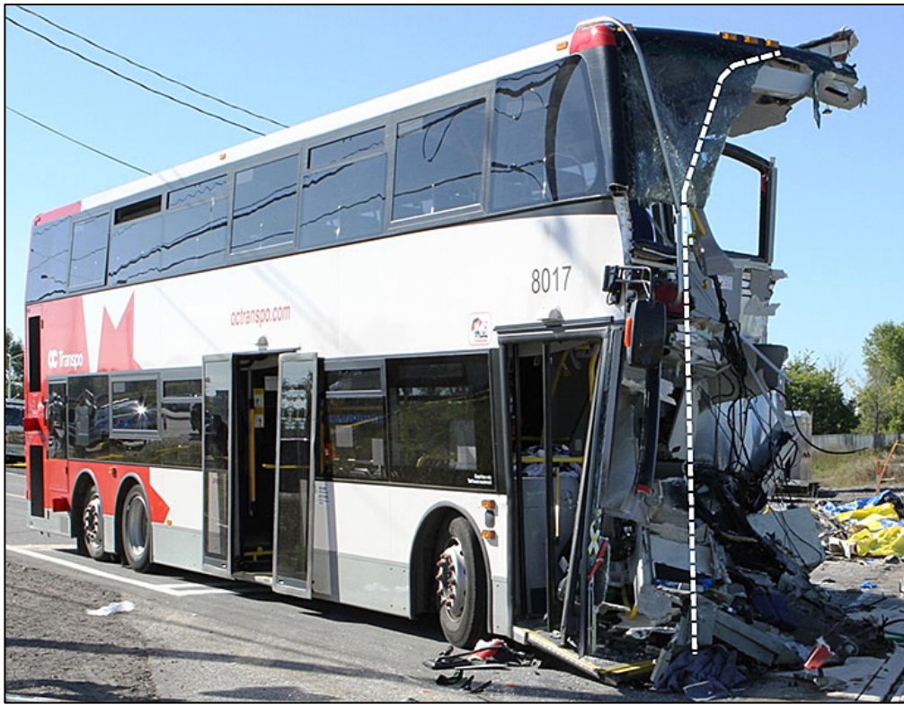
Photo 1. Right side view of the bus (the dotted line represents contour of locomotive VIA 915)
