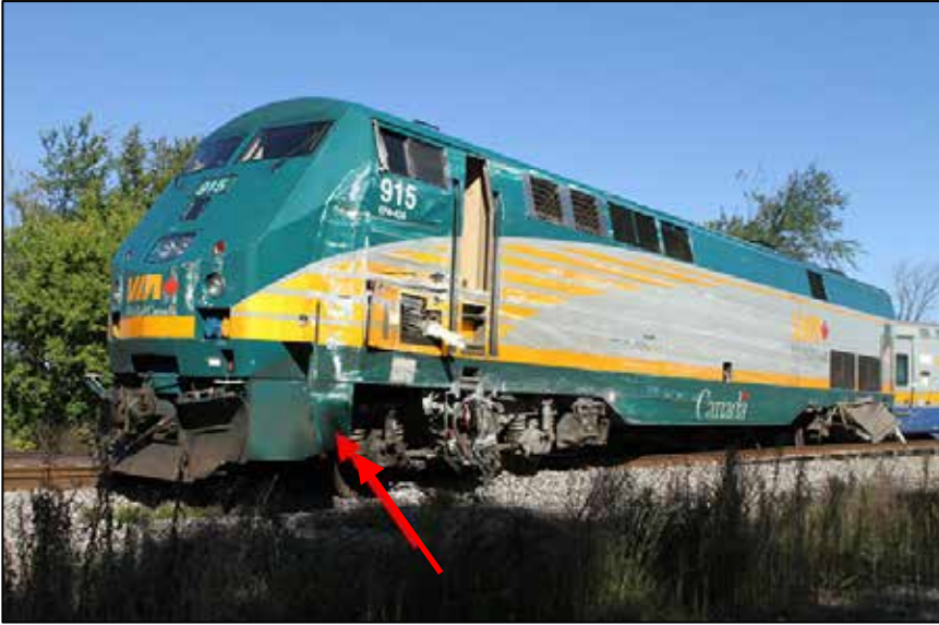
Photo 5. Damage on locomotive VIA 915
