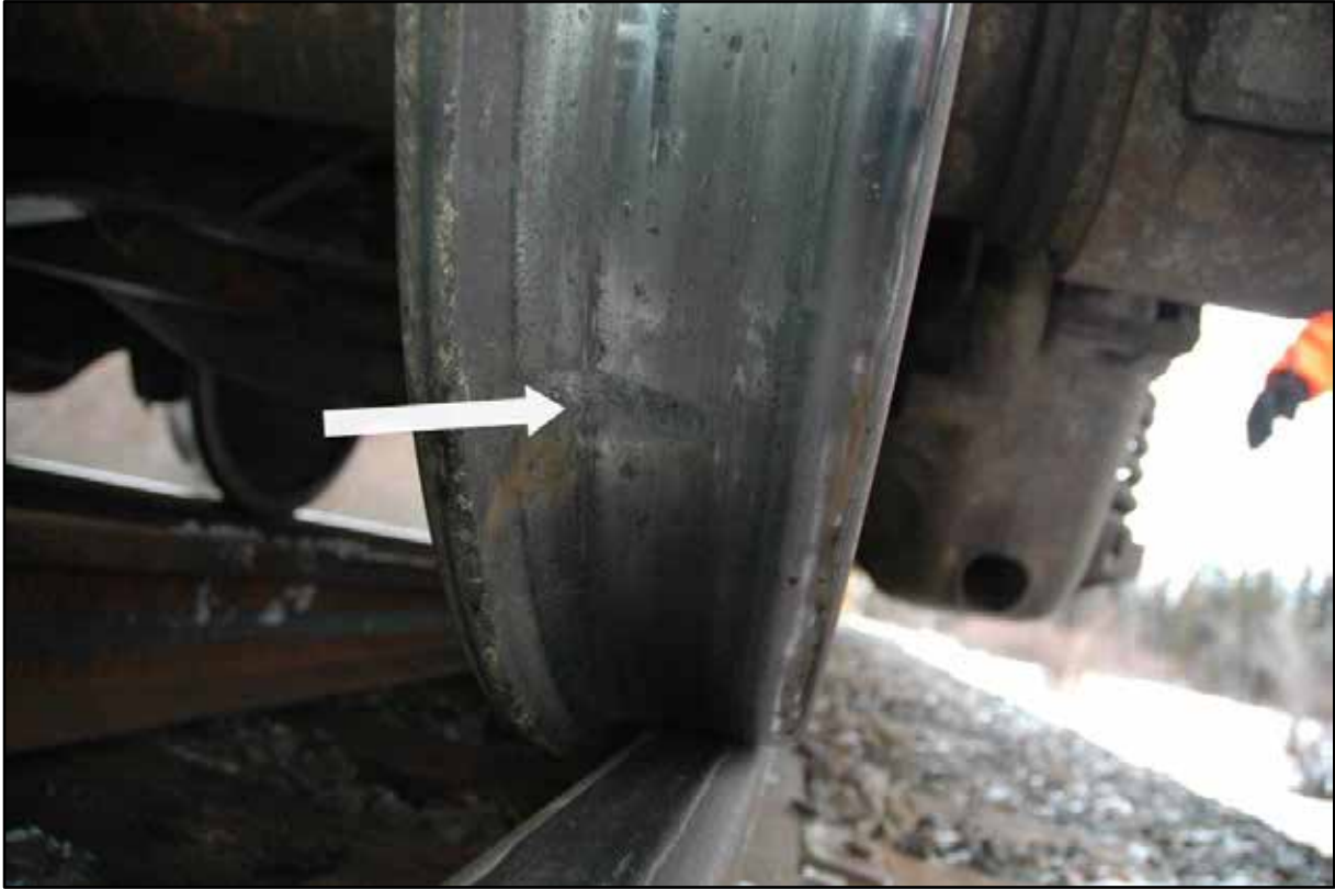
Photo 4. Wheel tread impact mark on car 38
