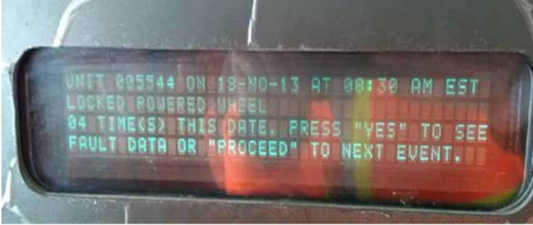
Photo 4. Human-machine interface display panel in SD60F locomotive (Source: Canadian National Railway)
