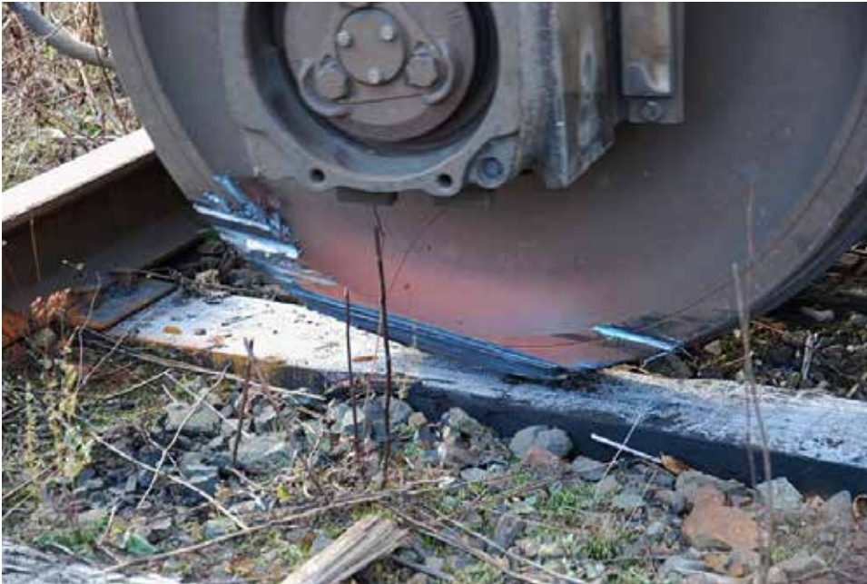
Photo 1. Rail burn damage
