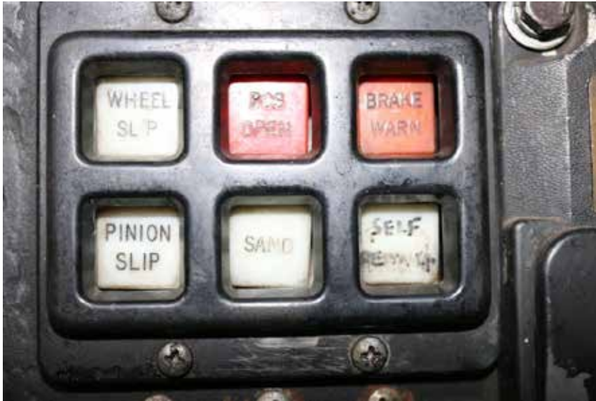
Photo 3. WHEEL SLIP indicator for SD60F locomotives
