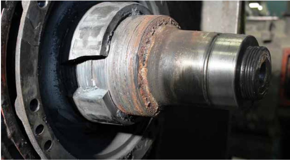
Photo 10. Close-up view of the inner ring during removal from the armature shaft
