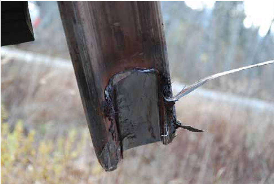
Photo 2. Damaged wheel tread
