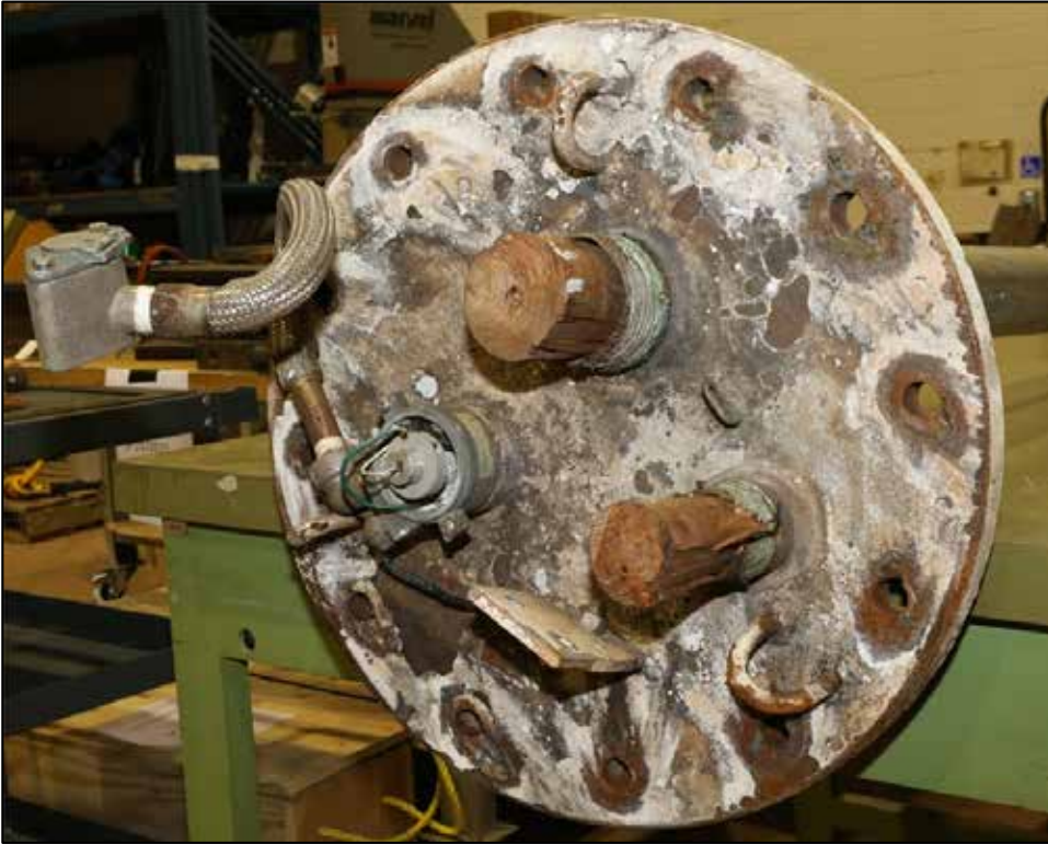
Figure 5. Top fitting assembly, wooden plugs are inserted at the valve locations where the liquid line and the vapour line were sheared off
