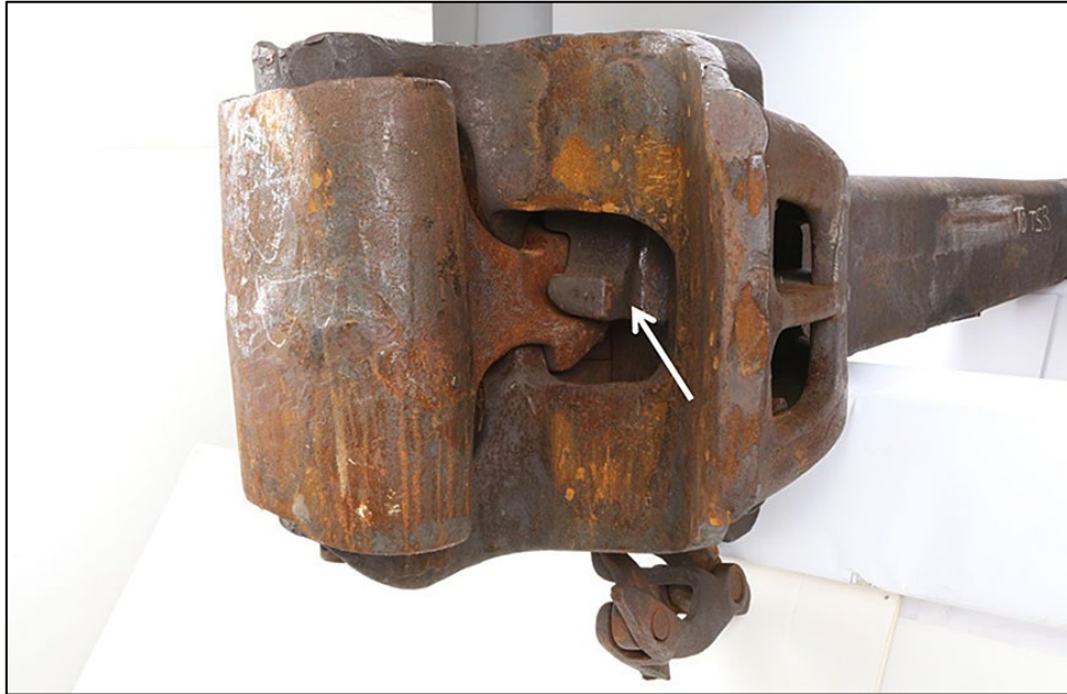
Figure 18. Locking block fully engaged
