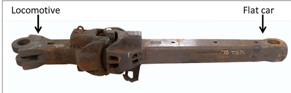
Figure 10. Locomotive CN 7506 and freight car CN 44257 coupler assemblies
