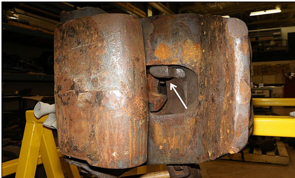
Figure 17. Lock-lift assembly toggle Z pin jammed in the locking block hole
