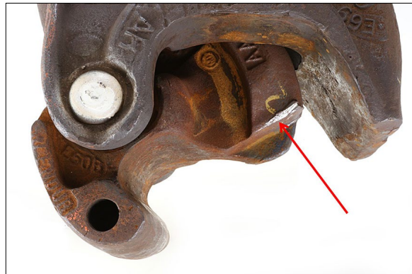
Figure 12. Top view of deformation on knuckle tail
