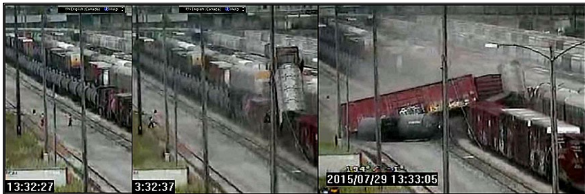
Figure 2. Sequential images from the Canadian National Railway Company (CN) yard video recording of the collision and derailment. The crew of train 422 approached the train then quickly evacuated the area just before the collision. (Source: CN)
