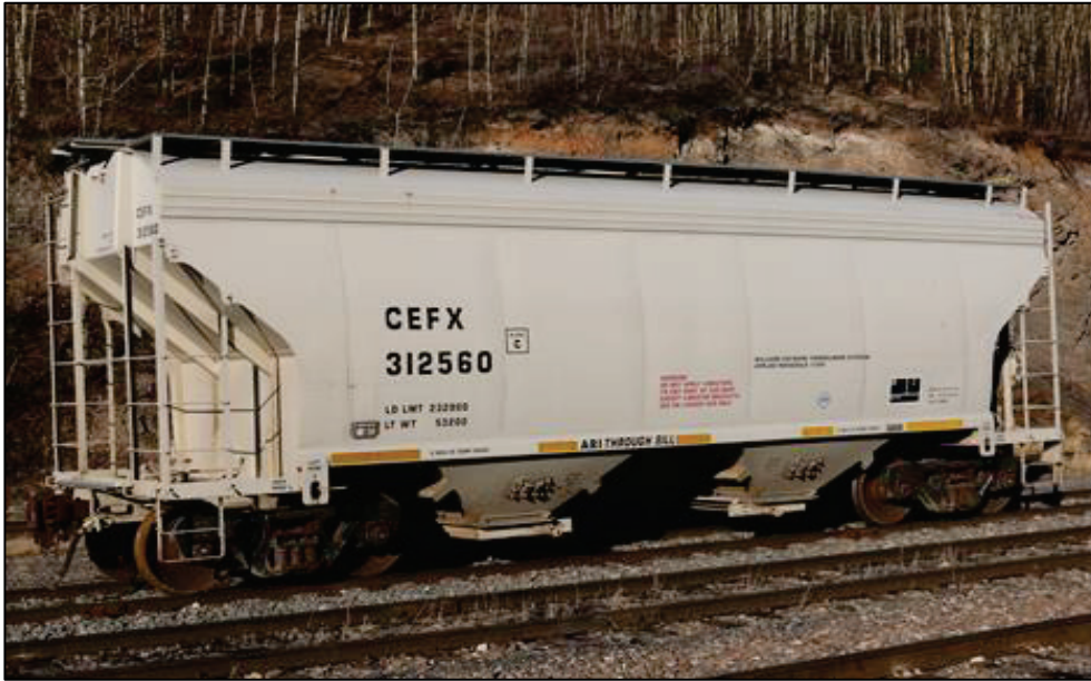
Figure 4. A typical 42-foot covered hopper car
