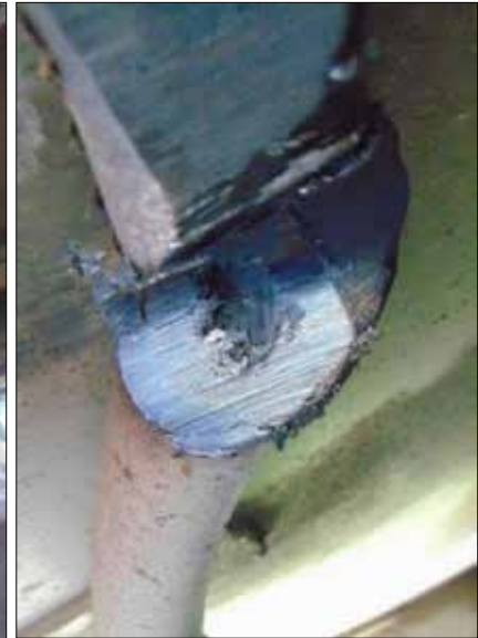
Figure 5. Close-up of air brake pipe burn/grind marks
