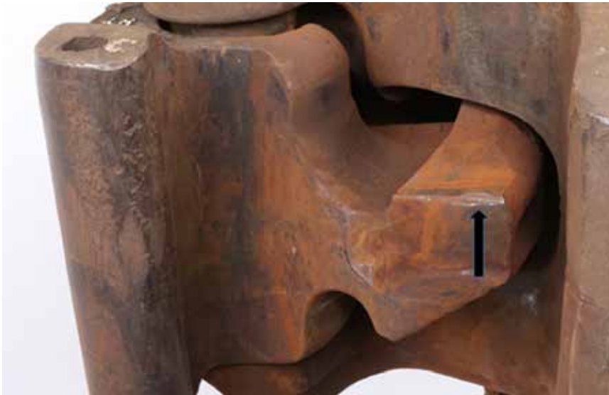
Figure 17. Knuckle of uphill car 1043, showing deformation on knuckle tail (indicated by an arrow)
