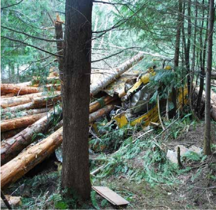
Figure 9. Second derailment location, showing the speeder buried under logs
