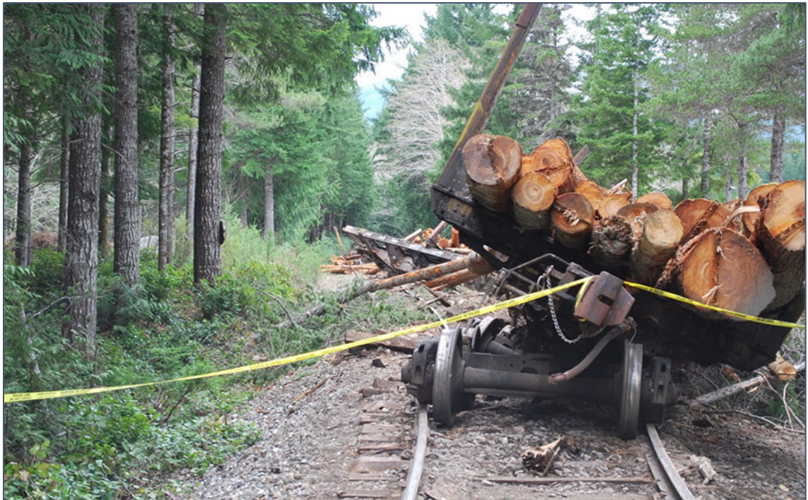
Figure 8. First derailment location, with derailed cars leaning or rolled to the high side of the curve
