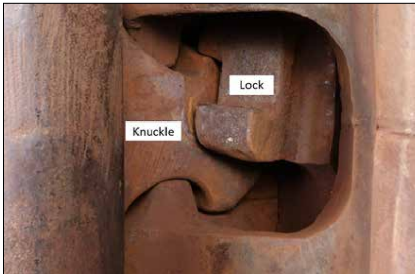
Figure 21. Subject coupler lock fully dropped and engaged with knuckle tail
