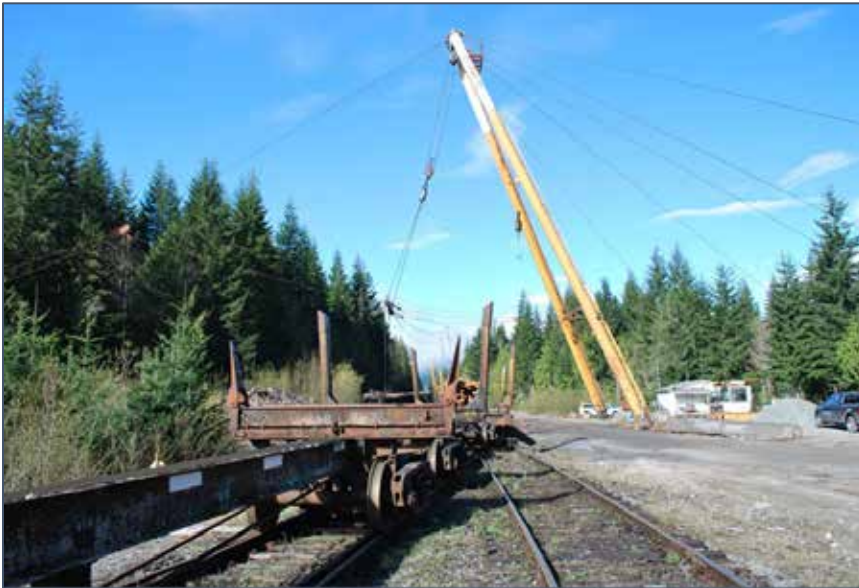
Figure 12. A-frame arrangement for unloading logs onto rail cars
