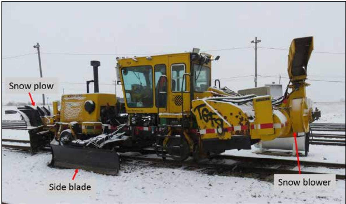
Figure 1. Track unit PNR 728
