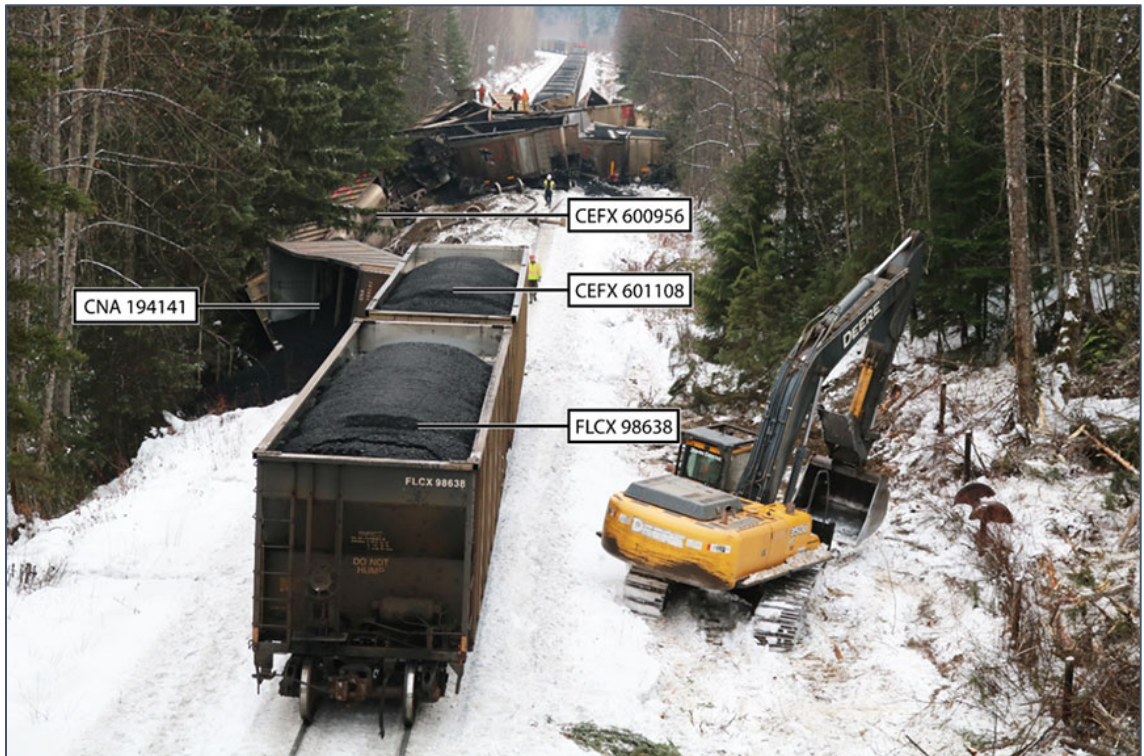
Figure 2. Eastward view of the derailed cars (Source: Interior News, with TSB annotations)
