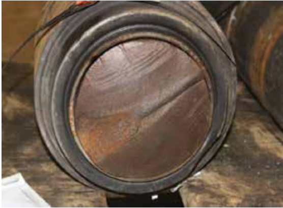
Figure 6. Mating fracture surface from the broken axle at the L1 bearing (view toward end of axle)
