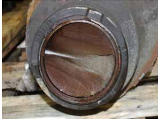
Figure 7. Mating fracture surface from the broken axle at the L1 bearing (view toward centre of axle)
