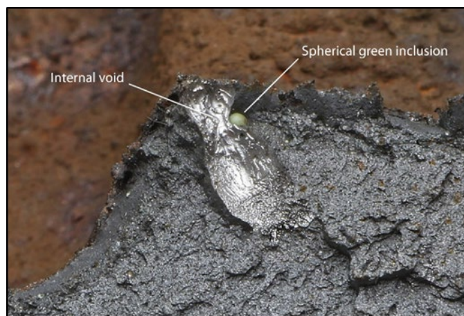
Figure 9. Photo of fracture face with spherical green inclusion and internal void (Source: TSB)
