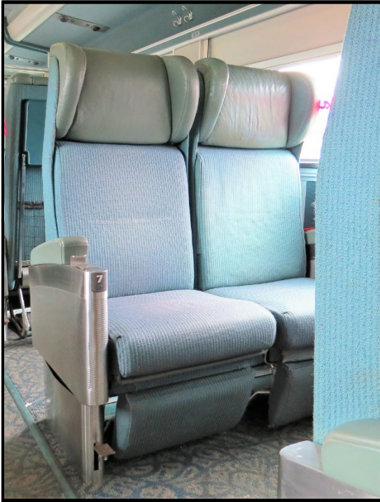
Figure 3. Seat 7B of car VIA 8147, with the legrest in the stowed position (Source: TSB)
