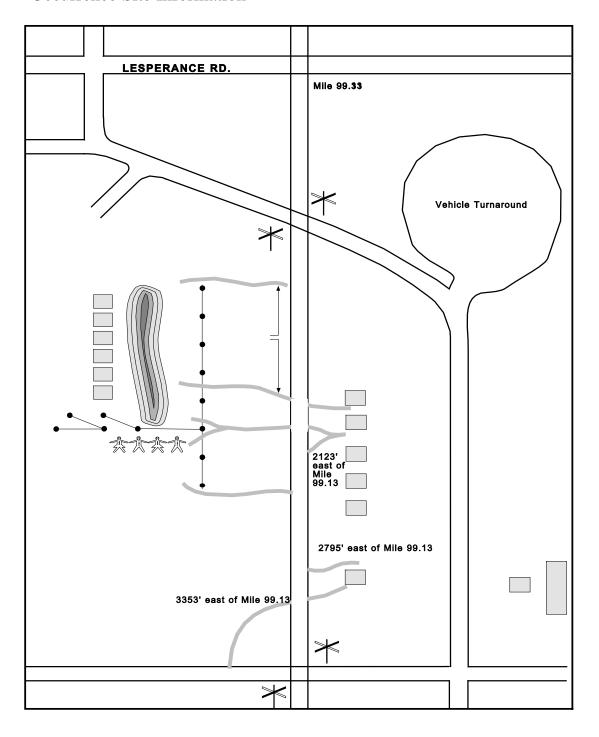
In the immediate vicinity of the occurrence site, the subdivision consisted of a single, tangent, east/west main track. Tecumseh Road intersects the main track at Mile 99.13 and turns east approximately one block north of the right-of-way. The road then parallels the main track, separated from the track by private lands. There were no barriers to restrict access to the railway right-of-way. Between Mile 99.13 and the Manning Road crossing,
